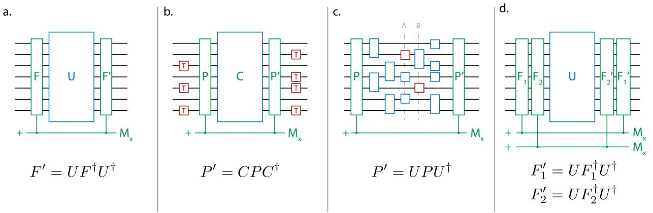
Our flag gadgets follow the same entangle-evolve-disentangle structure as the traditional flags used by Chao and Reichardt. They can detect any error which anticommutes with the F' operator, while leaving the logic of the circuit unchanged.
